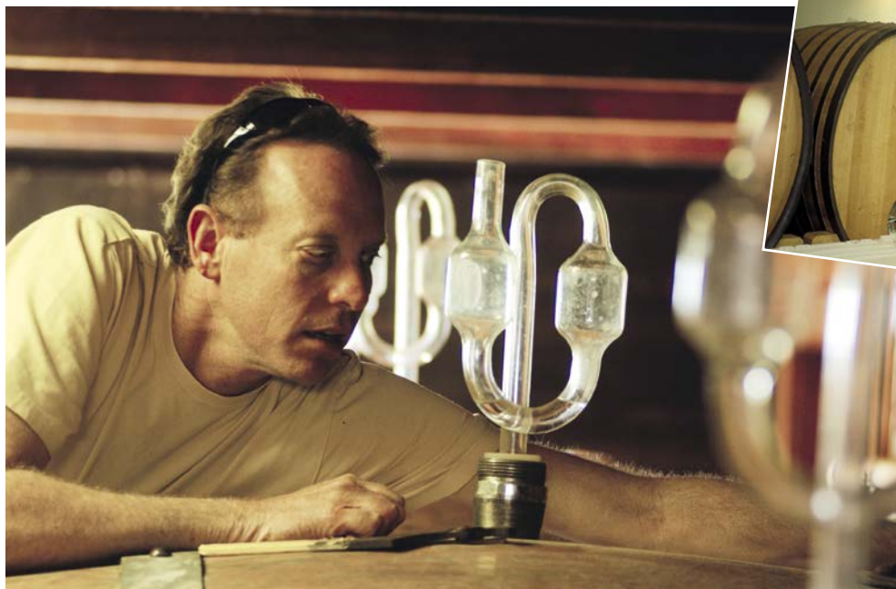
Jim Klein installing a “fermentation trap” on an oval during fermentation, which allows carbon dioxide to escape and keeps fruit flies out. Since some of the ovals are large, with capacities up to 1,500 gallons, the traps must also be large to accommodate the amount of gas being generated.
