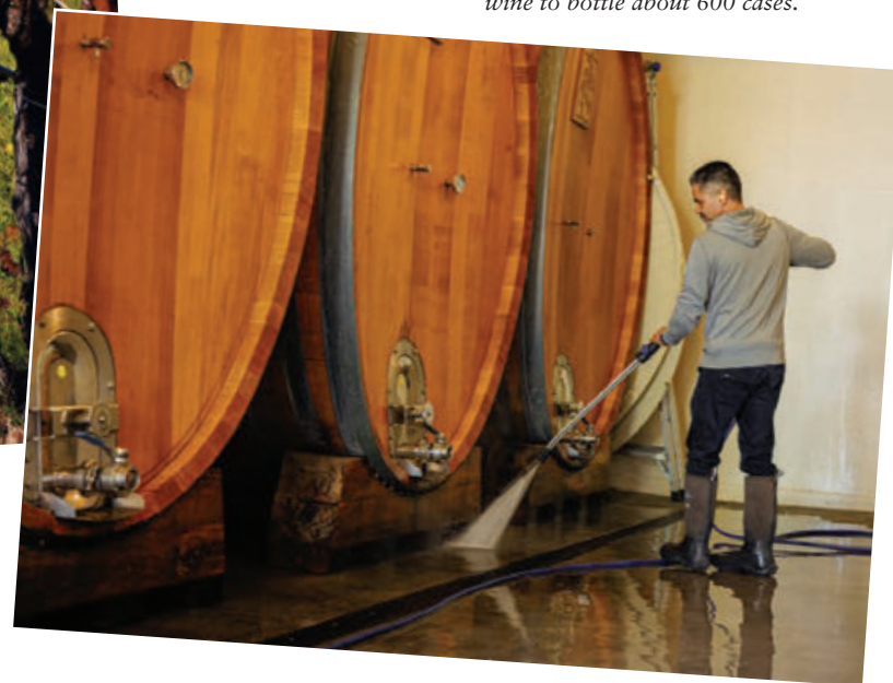
Pressure washing the floor prior to harvest. These larger ovals hold enough wine to bottle about 600 cases.
