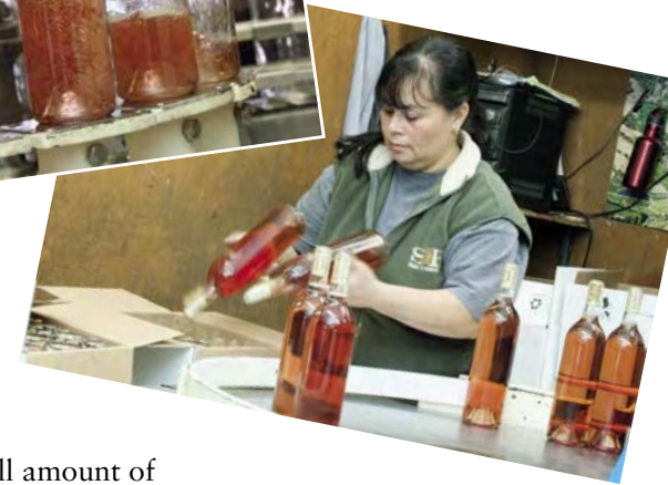
After the cork is inserted, the bottles are left upright for a little while, then Josephina Eligio packs them neck down. We prefer to label later; that way we can examine each bottle to make sure there are no "leakers" or other problems.
